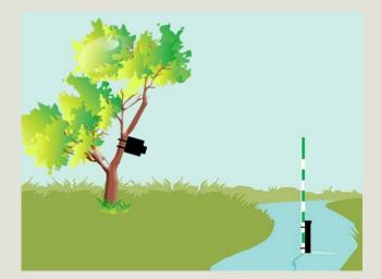
SRP Flowtography units are stand-alone and solar-powered and collect images of event gages located within stream channels and their immediate surroundings.
